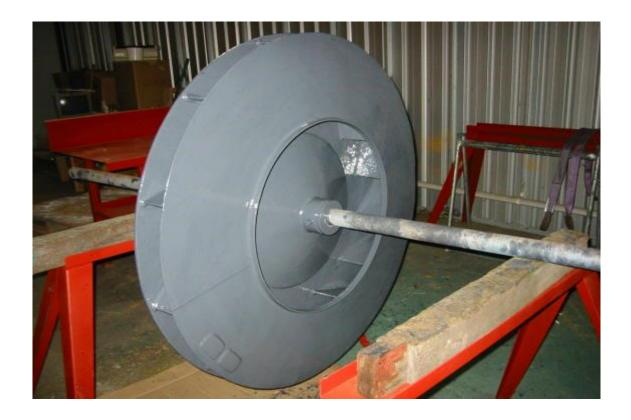
For more arduous conditions alumina ceramic tiles can be bonded to the fans and housings to enhance the service life of components. The use of high shear strength epoxy structural adhesives ensures the small tiles  $(10 \times 10 \times 2 \text{ to } 4 \text{ mm})$  are securely attached to the equipment.
